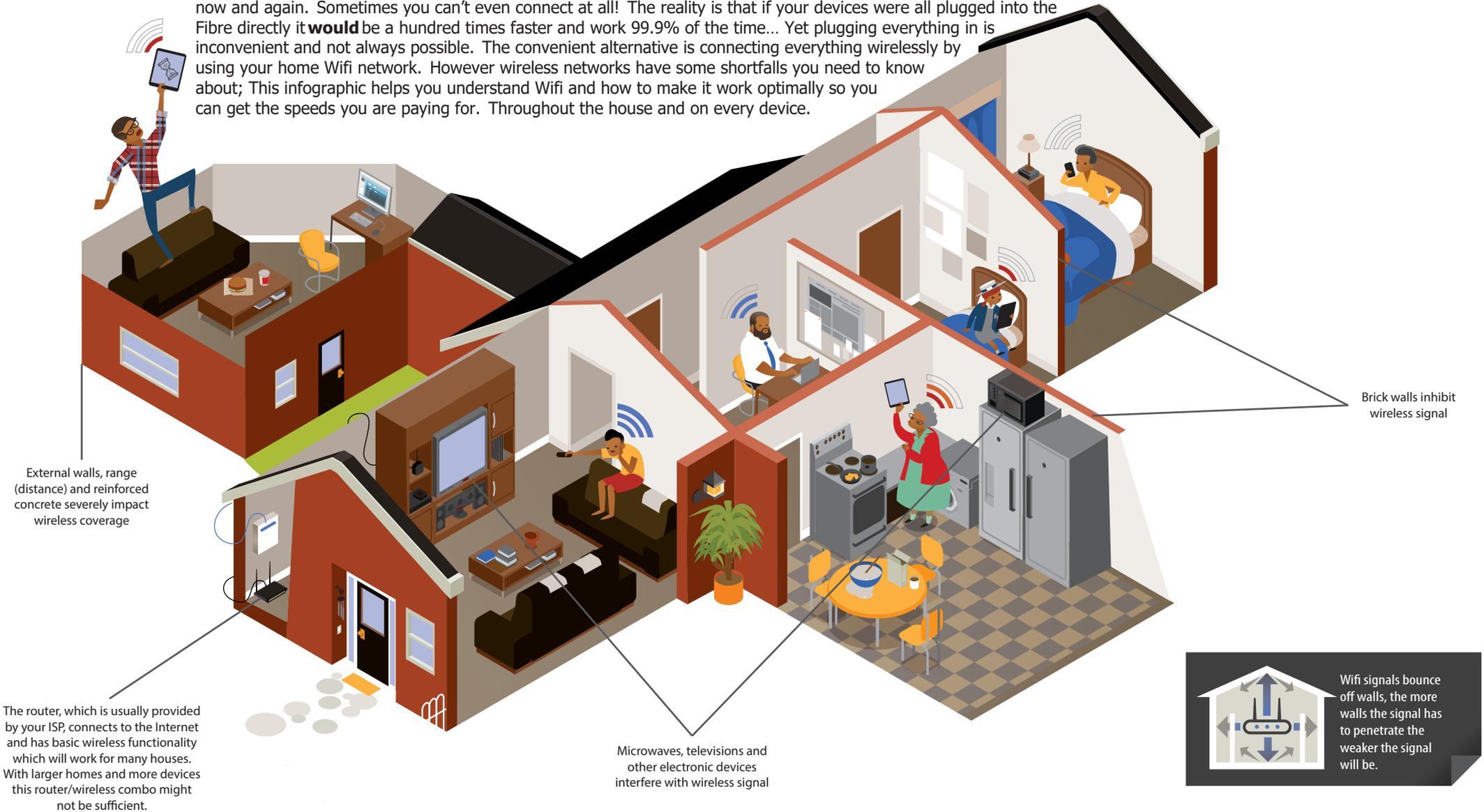
External walls, range (distance) and reinforced concrete severely impact wireless coverage
